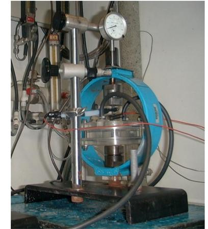
Machine stress corrosion: Carnots IFPEN
